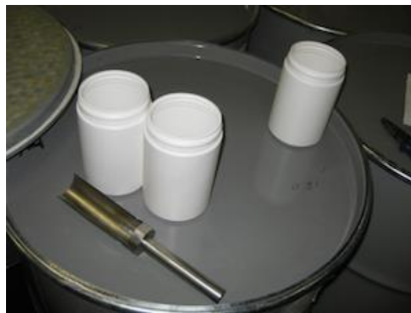
Figure : Sample collecting Equipments (Sampling trowel and Plastic bottles, wide opening, not transparent)
