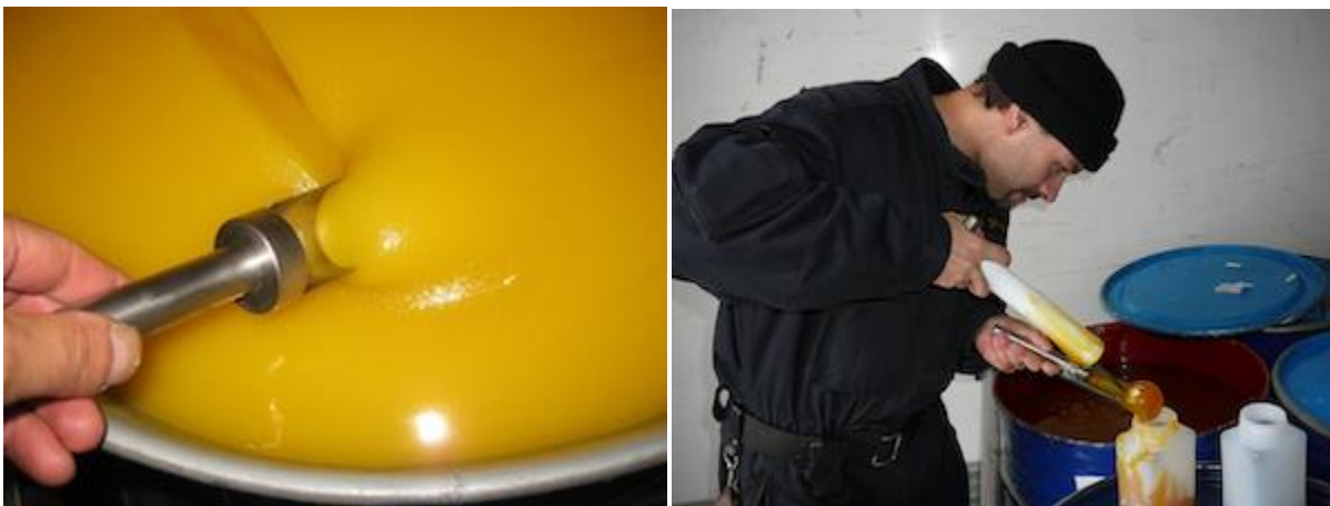
Figure : Samples taken by Piston-tube sampler into rectangular plastic bottles, size 500 ml with leak-proof or air tight closure
